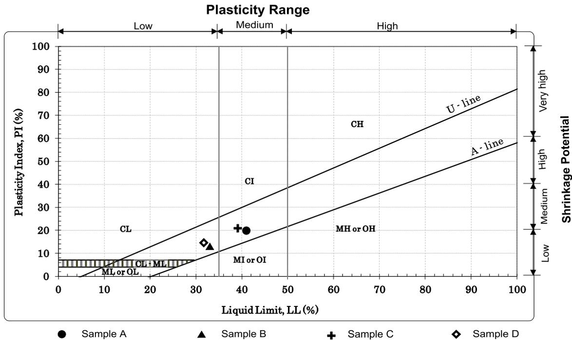
Figure 2. Plasticity chart for the soil samples (After Casagrande, 1948)
